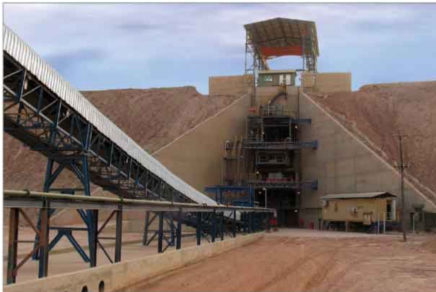
Figure 28: Typical Dumping Station
